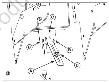
Figure 10. Catcher Alarm Adjustment
